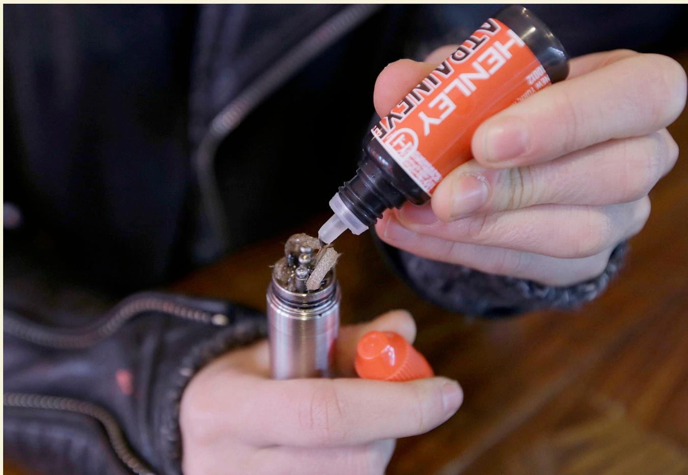
Although manufacturers offer many different designs of e-cigarettes, all involve the same basic concept: A heating element at one end aerosolizes a liquid nicotine solution, and the vapor is inhaled through a mouthpiece. © AP Photo/Frank Franklin II
